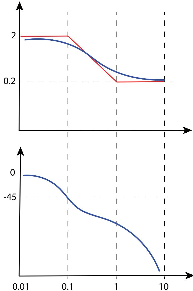
b) The input is given as  $u(t) = 10\sin(t)$ . We need to find the magnitude and phase of the sinusoidal transfer function at  $\omega = 1$ .
